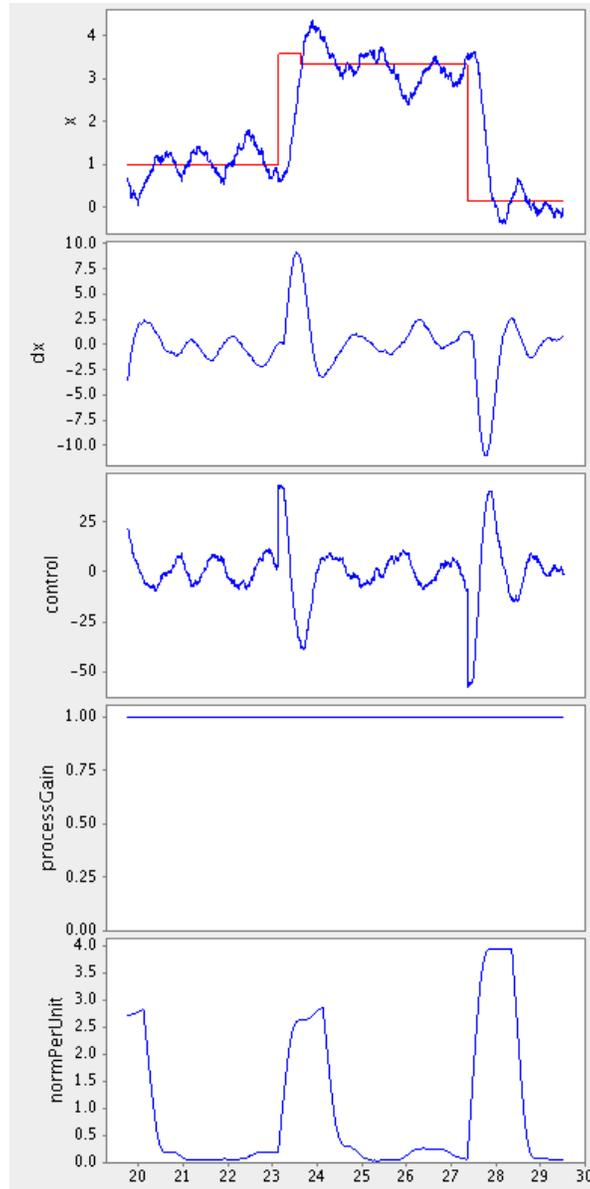
Figure 1: The system with the process gain fixed to unity being run with a PID controller with  $K_P = 15$  and  $K_D = 5$  (which is not the best possible one). From top to bottom the graphs show the current location (including the setpoint with red), the velocity, the control signal, the process gain, and finally the integral of the norm in the previous one time unit (which is useful for debugging but not for evaluating the systems - for that, the integral must be taken over all time).
